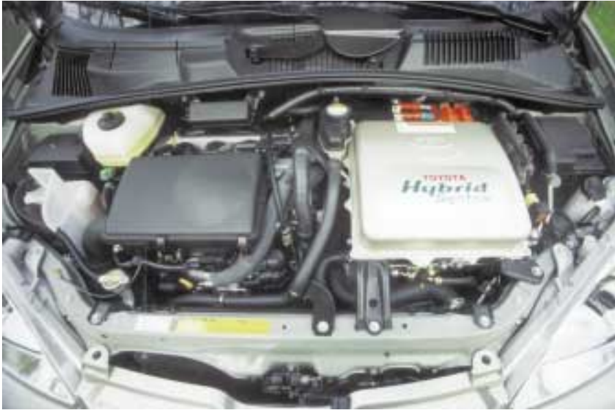
Under the hood—the gasoline engine and electric motor/charger.
